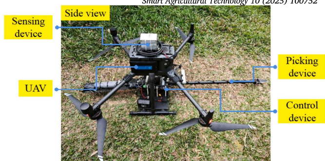
Fig. 1. Distribution of Hardware Modules for Longan FP-UAV.
