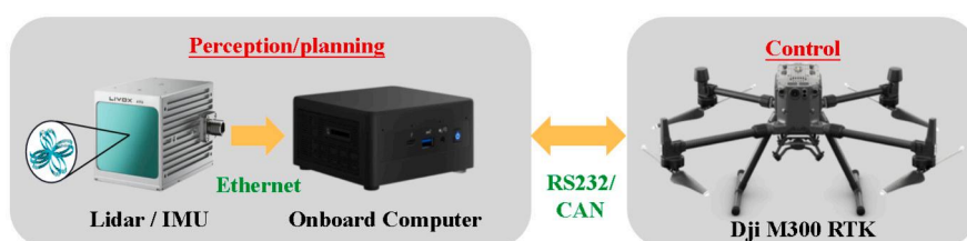
Fig. 3. Information transmission process of the FP-UAV.
