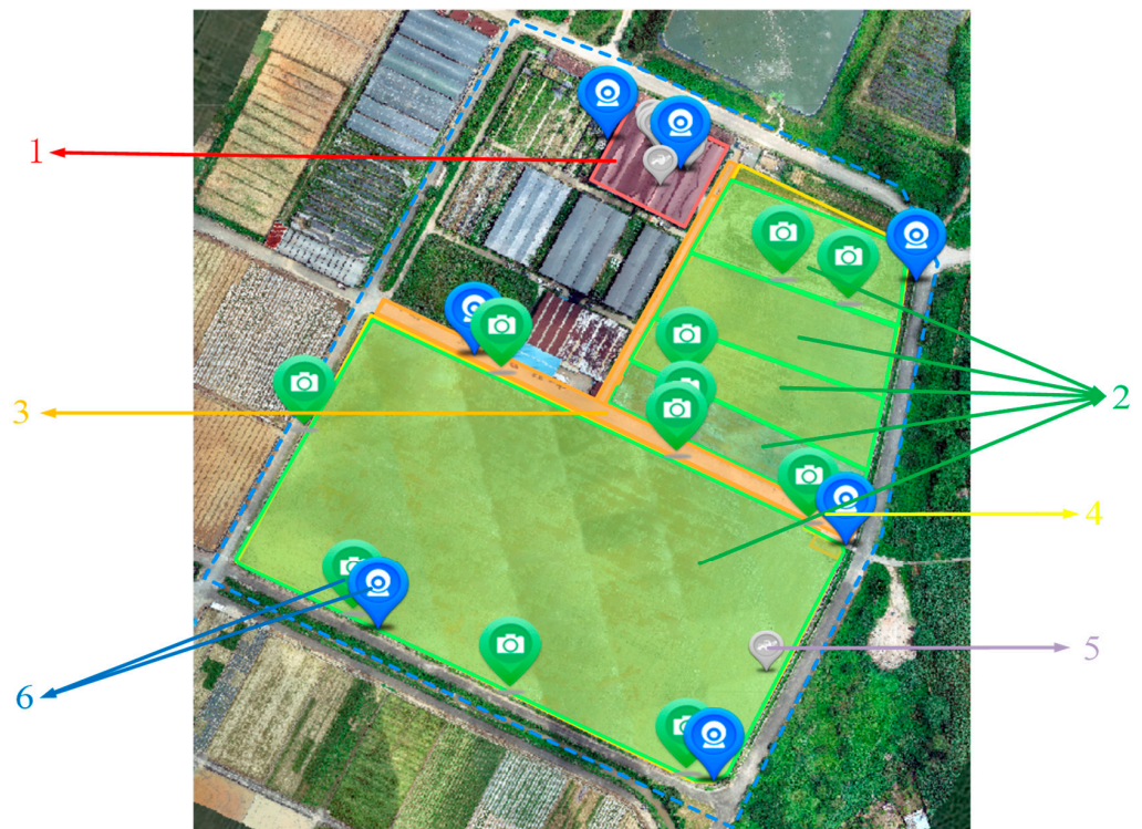
Figure 14. Constructed map of unmanned farms. Note: 1. Hangars. 2. Fields. 3. Roads. 4. Obstacles. 5. Farm machinery. 6. Sensors.
