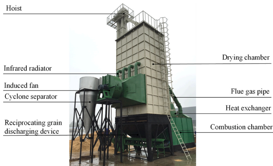
Fig. 1. Diagram of 5HP-20 industrial-scale circulation counter-flow paddy dryer.
