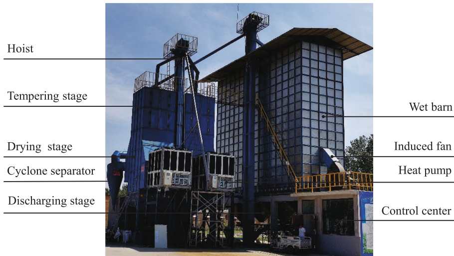
Fig. 1. Diagram of 5HP-50-CLHP wheat dryer.
