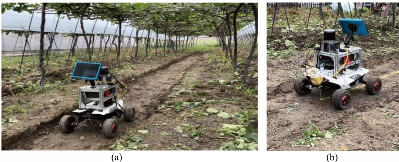
Fig. 11 Test site grape fields a robots conduct field test, b the yellow sand grains record the movement path of the robot during navigation
