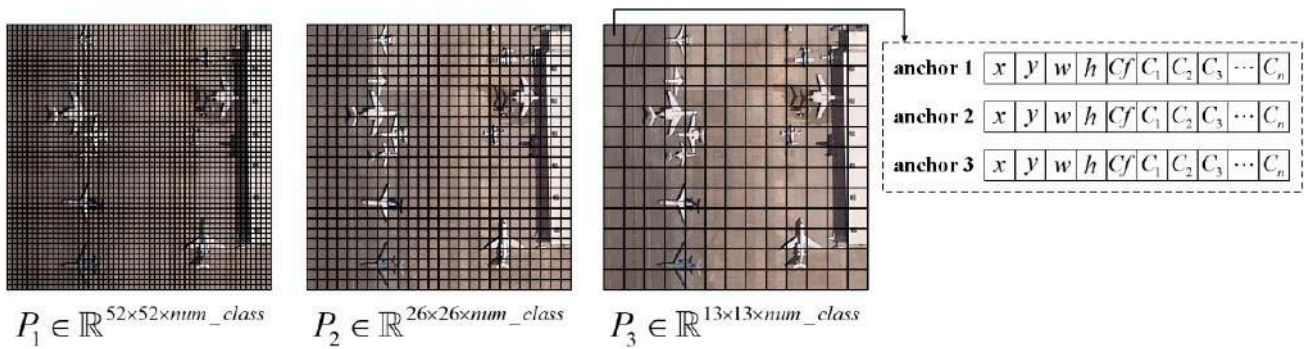
Figure 8. The image is divided into 52 \times 52 , 26 \times 26 and 13 \times 13 by P_1 , P_2 and P_3 , respectively.
